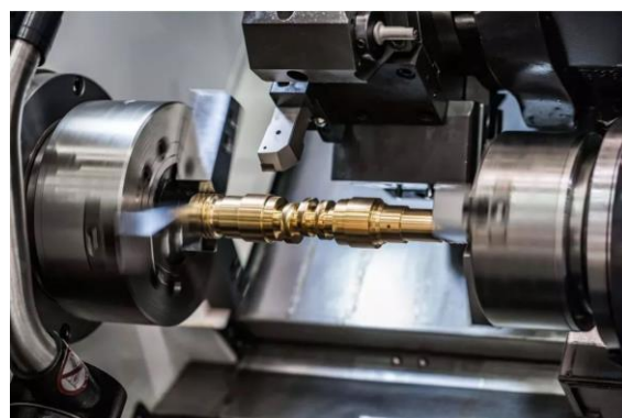
Figura 1.5. Strung orizontal prelucrând un ax cu came – Copyright ©2021 EKO Group. All Rights Reserved. [8]
