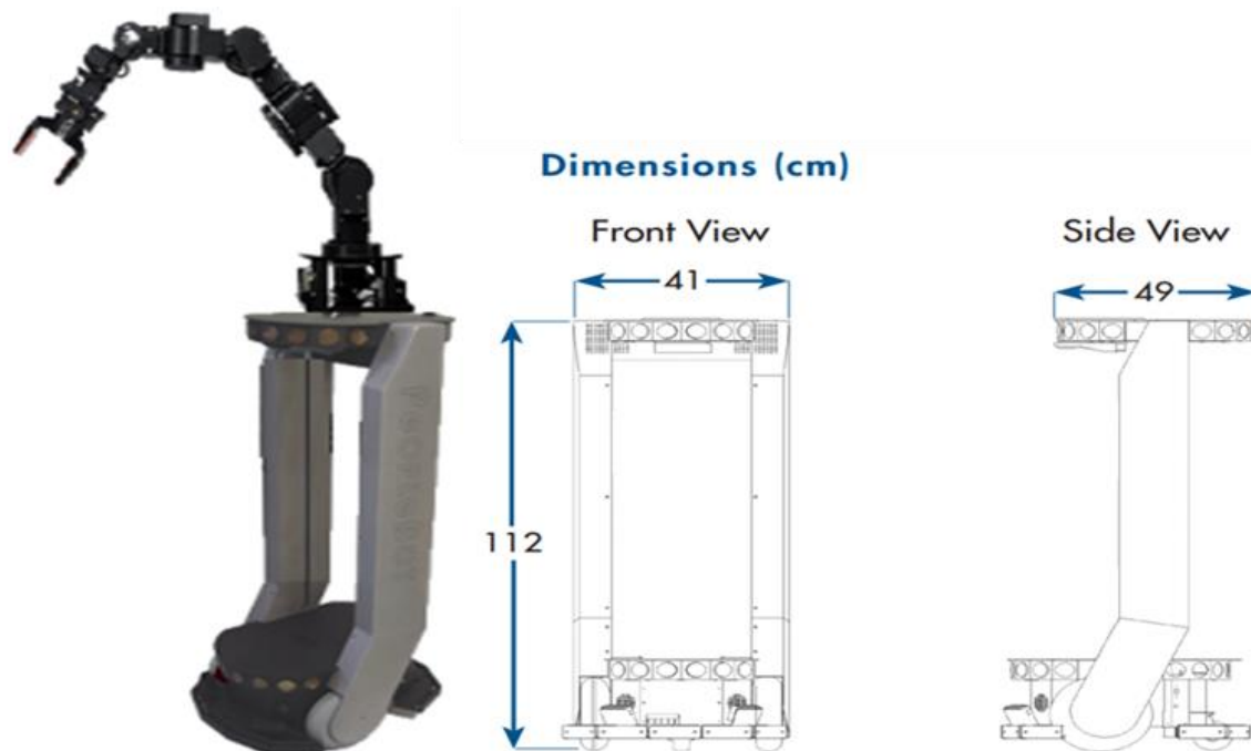
Figura 3. PeopleBot WMR cu braț robotic Cyton cu 7 grade de libertate (7-DOF).
